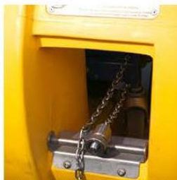
Rear of swing shows wheel lock chains which extend around wheelchair wheel, are pulled taut and fastened to the lock.
